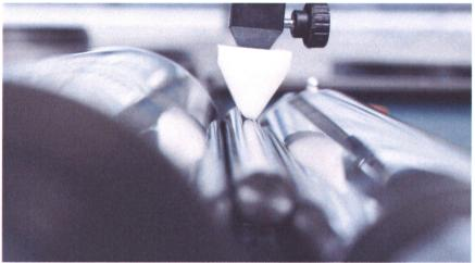
to the workpiece. There is a version with two sets of working rollers of 150 mm for shorter workpieces and a version with one set of rollers sized at 500 mm for longer workpieces. Both are available with a manual pressure device for variable pressure application. This enables the user to decide where pressure should be applied and material should be taken off. Through this
